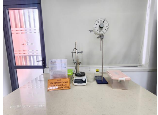
Device: Determining the Surface Tension of a Liquid by the Ring Method
